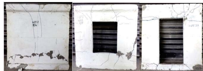
Fig. 13 Crack Patterns of UHPFRC wall panels
